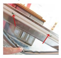
Open the drawer and pull off the seal at the upper edge. Underneath or behind the seal are the screws that fix the handle.
