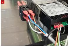
1 Open the door of the cooling machine compartment and 2 disconnect the cables from the switch
