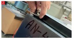
With the door closed, loosen the 3 screws and 2 pull the hinge out upwards.
